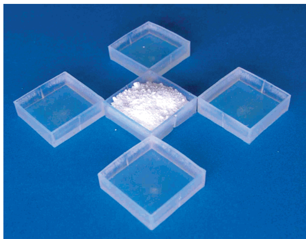
Figure 5. Processed samples of PBA 37 /PS 63 (BS2) at 25 °C under 34.5 MPa for 1 min. Middle box contains original dry powder as obtained from polymerization.
